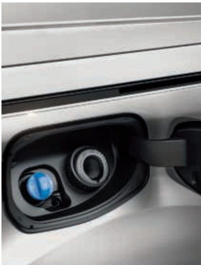
Ford Easy Fuel capless refuelling system (Standard)
